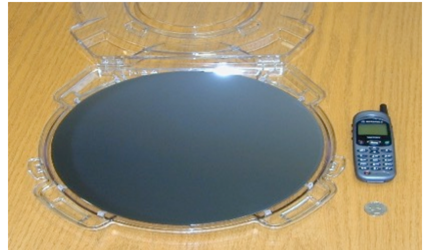
GaAs on 300 mm Silicon using MBE
