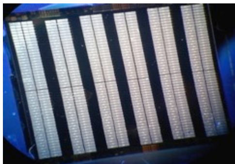
Chip showing 300 DFB lasers with yield >95%
