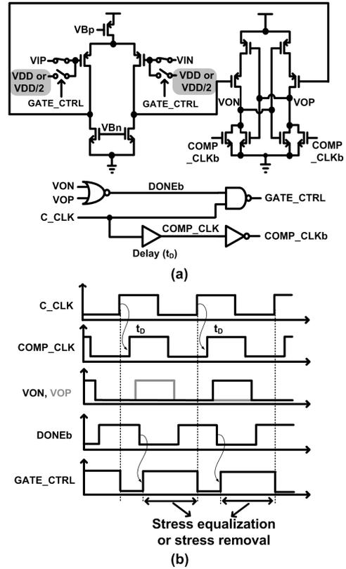
Fig. 5. (a) Schematic and (b) timing diagrams of comparator circuit consisting of a pre-amp stage and a latch circuit [8]. Additional switches are used for the proposed stress equalization and stress removal techniques.
