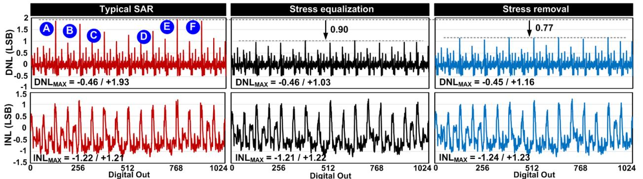
Fig. 6. Measured DNL (top) and INL (bottom) using the proposed techniques compared to a typical SAR ADC. Measured data from a 65nm test chip shows a DNL improvement of 0.90 and 0.77 LSB using stress equalization and stress removal, respectively. The impact on INL was negligible.
