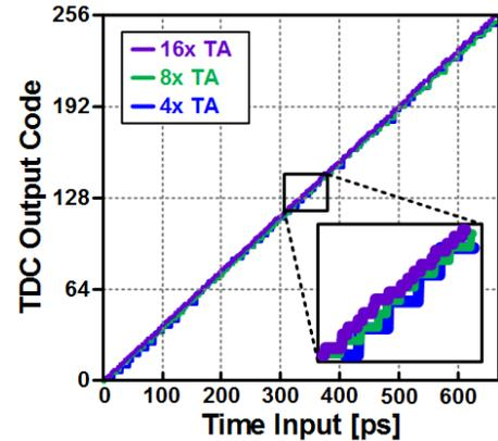
Fig.8. Measured TDC output with respect to a ramp time input.
