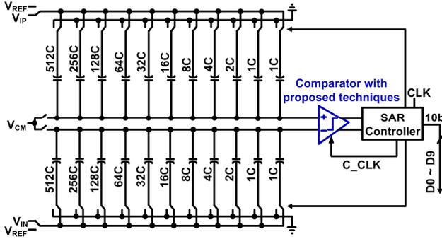
Fig. 4. Block diagram of a 10-bit differential charge-redistribution SAR ADC. The proposed stress mitigation techniques are implemented in the comparator circuit block.
