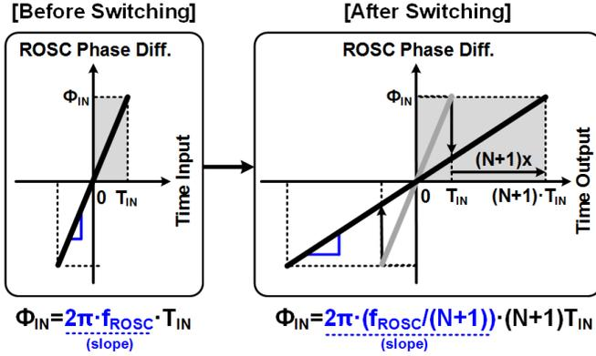
Fig.2. Switched ring-oscillator based time amplifier mechanism.
