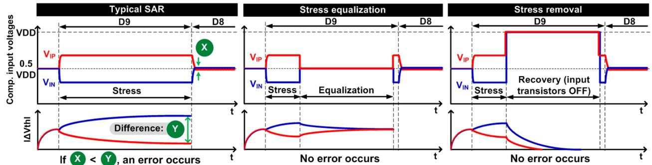
Fig. 3. Illustration of proposed stress equalization and stress removal techniques compare to a typical SAR ADC. Comparator input voltages (top) and corresponding  $V_{th}$  shift (bottom) are shown for just the first D9 conversion step here for simplicity. By either equalizing the input voltages or connecting them to  $V_{DD}$  right after the conversion, the comparator input offset due to asymmetric voltage stress can be minimized in the next conversion step.
