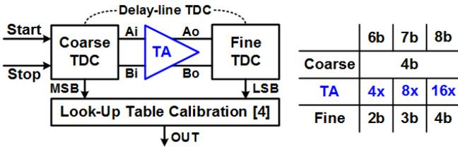
Fig.6. Two-step TDC circuit block diagram.
