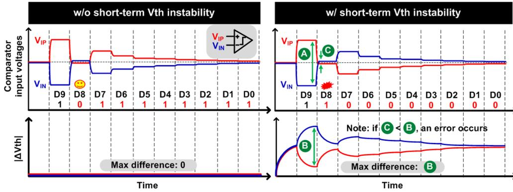
Fig. 2. Comparison of 10-bit SAR ADC operation without and with BTI induced short-term  $V_{th}$  instability. Comparator input voltages (top) and corresponding  $V_{th}$  shifts (bottom) for P-type input transistors are shown for each SAR conversion step. Comparators with N-type input transistors are equally susceptible to short-term  $V_{th}$  instability issues due to PBTI in high-k metal gate technologies.
