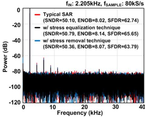
Fig. 8. FFT for a 2.205kHz differential sinusoidal input sampled at 80kS/s. Improvements in SNDR, ENOB, and SFDR using the proposed techniques can be seen.
