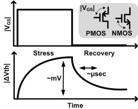
Fig. 1. Illustration of short-term  $V_{th}$  degradation and recovery in a CMOS transistor due to Bias Temperature Instability (BTI).
