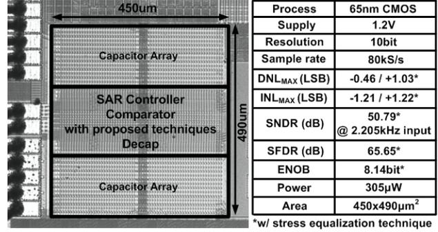
Fig. 9. Die photo and performance summary table of the 65nm SAR ADC test chip with the proposed techniques.
